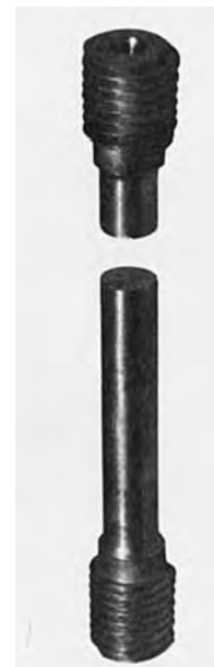
Photo 2.5 Tested specimen of a brittle material.
