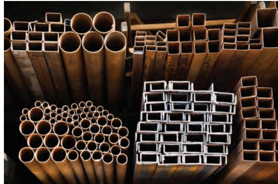
Photo 6.3 Box beams and tubes.
