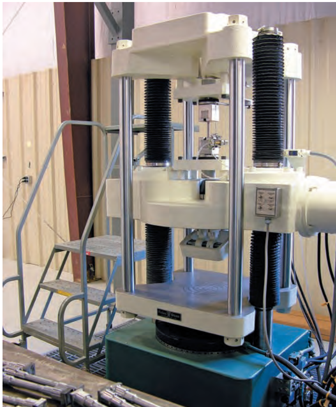
Photo 2.2 This machine is used to test tensile test specimens, such as those shown in this chapter.
