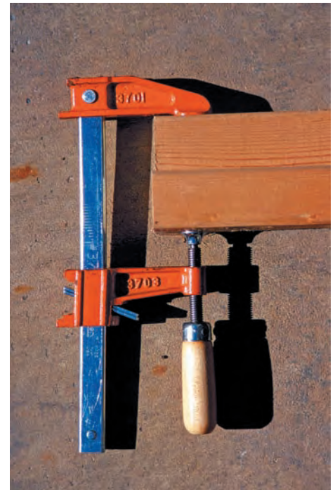
Photo 4.2 Clamp used to glue lumber pieces together.
