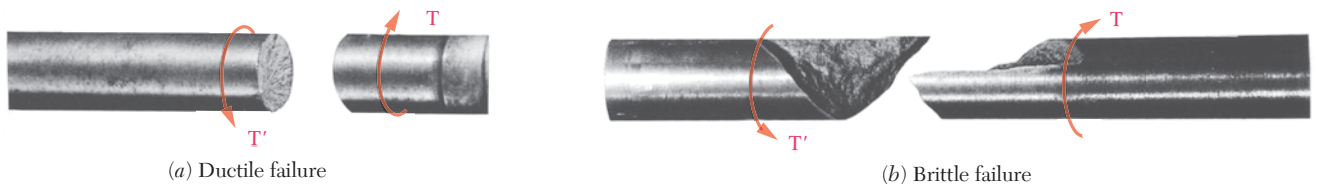
Photo 3.2 Shear failure of shaft subject to torque.
