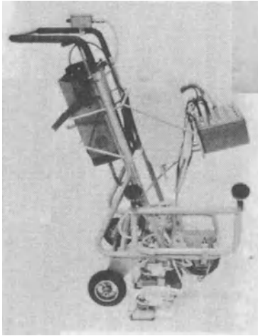
Fig. 24.3. Five-channel plate tester (design Krautkrämer)
