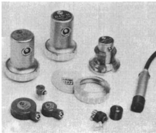
Fig. 10.30. A selection of vertical probes: top and bottom left with hard facing-layer; top centre with exchangeable wear-resistant film; lower right with exchangeable delay line, and with cast-resin face for immersion techniques
