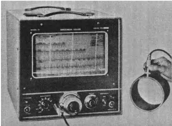
Fig. 11.15. Branson Vidigage, model 14, showing the wall-thickness measurement of 4.2 mm steel
