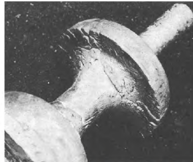
Figure 5.1 Cold laps and shut in a steel casting (courtesy of Institute of British Foundrymen)
